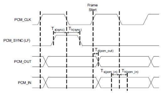
Figure 8-4: PCM interface timing diagram (master)
