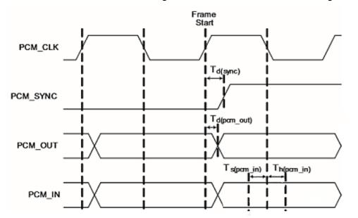
Figure 8-3:PCM interface timing diagram (slave)
