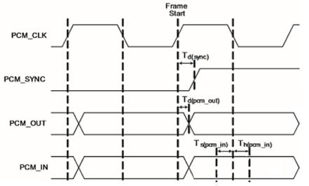
Figure 10-3:PCM interface timing diagram (slave)
