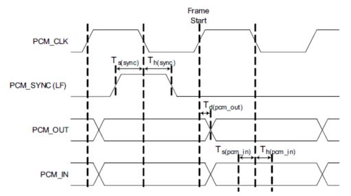
*Figure 10-4: PCM interface timing diagram (master)*
