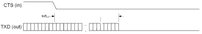
Figure 10-1: HCI UART transmit flow control timing
