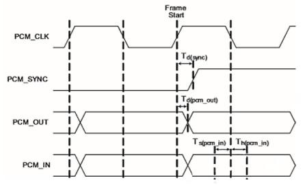
Figure 10-3:PCM interface timing diagram (slave)
