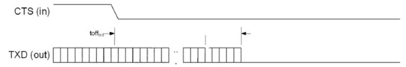
Figure 10-1: HCI UART transmit flow control timing
