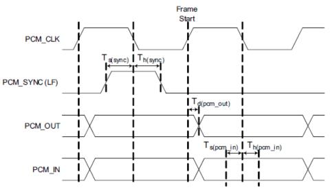
Figure 10-4: PCM interface timing diagram (master)
