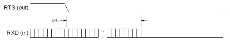
Figure 10-2: HCI UART receive flow control timing
