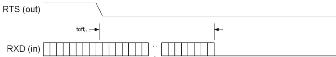
Figure 8-2: HCI UART receive flow control timing
