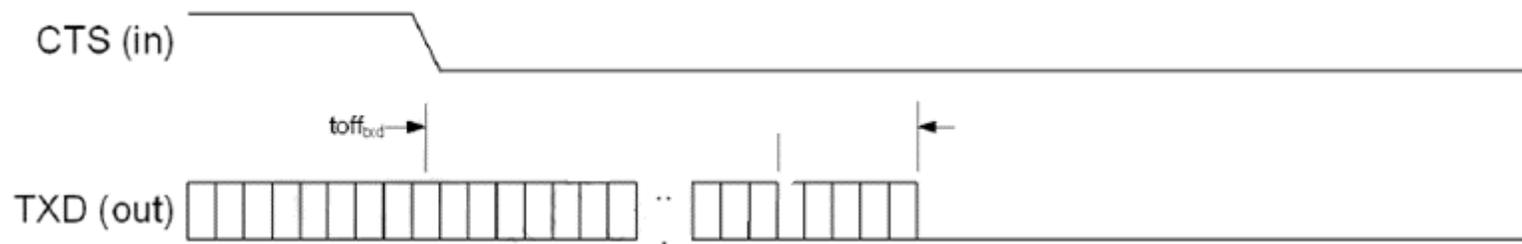
Figure 8-1: HCI UART transmit flow control timing
