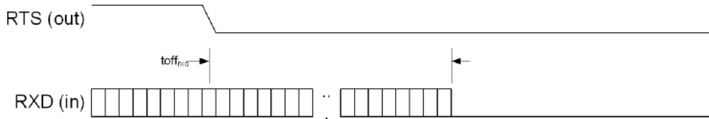
Figure 8-2: HCI UART receive flow control timing
