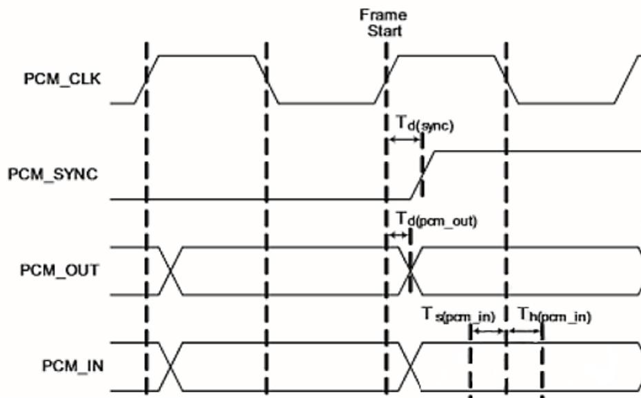
Figure 8-3: PCM interface timing diagram (slave)
