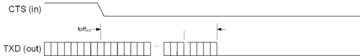
Figure 10-1: HCI UART transmit flow control timing
