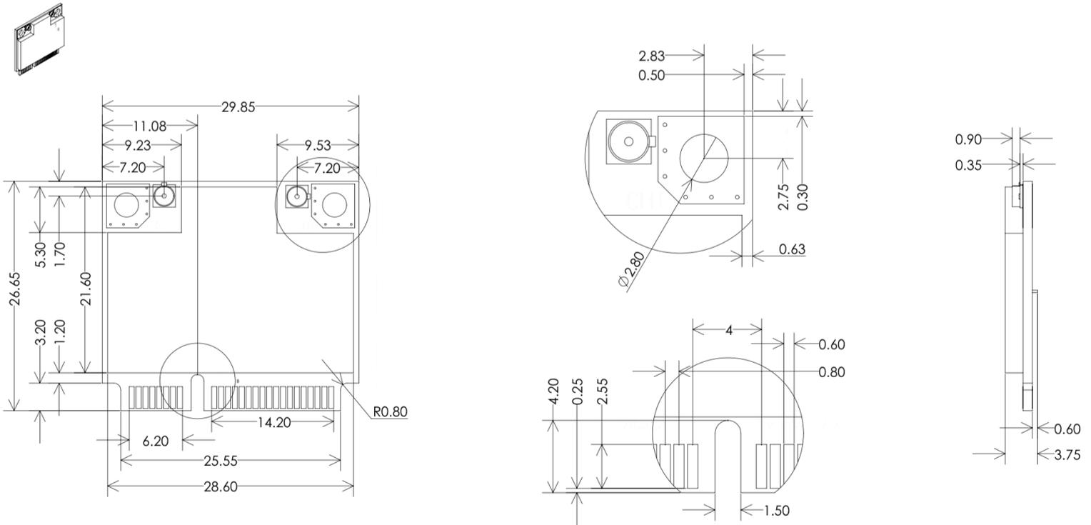
\* Measures in millimeters (mm). Tolerance below 0.15mm unless otherwise specified.
